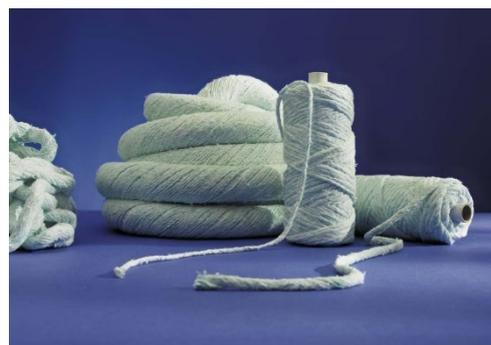
Ecomab® Twisted Rope is reinforced with glass or metal wire and contains approximately 20% organic carrier fibre to facilitate the carding process. The carrier fibre burns out at a low temperature, but this has no effect on the properties of the speciality glass fibre.
