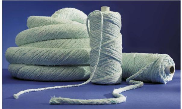
Keramab® twisted rope is reinforced with glass (or metal wire and contains approximately 20% organic carrier fibre to facilitate the carding process. The carrier fibre burns out at a low temperature, but this has no effect on the properties of the ceramic fibre.
